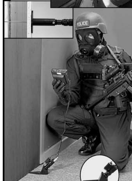
The Under-Door Scope slides under doors in less than a quarter of an inch of space.
