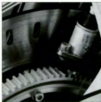
Front and rear toothed sensors are constantly monitored by an electronic control unit to determine when intervention by ABS is necessary.
