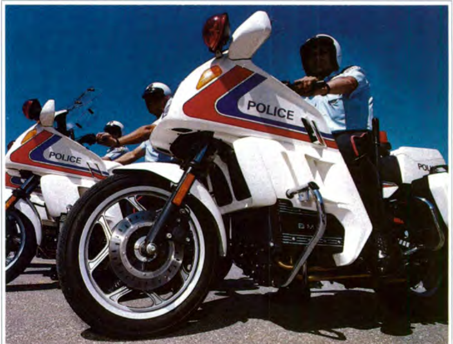
The BMW K100LT. The police motorcycle incorporates the ABS system designed to give the officer more control in any road conditions, from dry pavement to rain, sleet, sand or oil patches.
