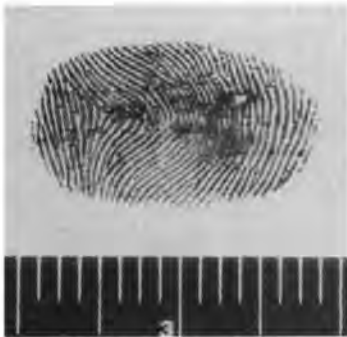
The original photograph of this picture showed white ridges on a dark background. A police photographer copied the image with PolaPan, then printed the PolaPan slide onto conventional photographic paper to reverse the print.
