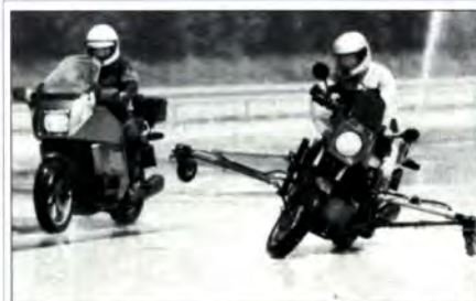
The outtrigger-equipped motorcycle, without ABS, has locked up the wheels and lost stability during hard braking on wet pavement (right). The ABS-equipped bike remains upright and controllable under the same conditions (left).
