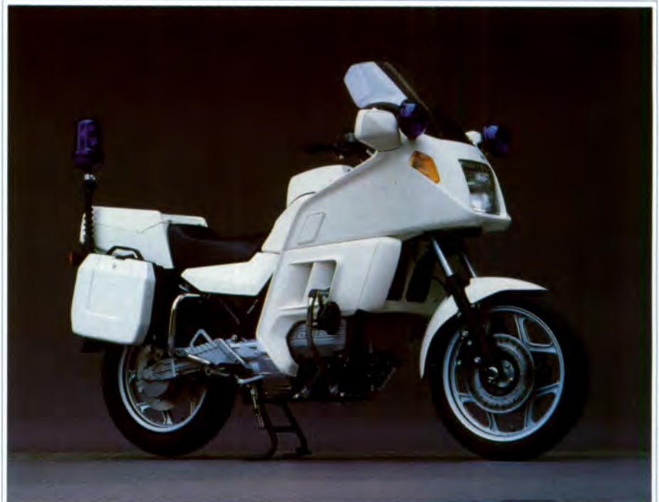
The BMW K100LT: The police motorcycle incorporates the ABS system designed to give the officer more control in any road conditions, from dry pavement to rain, sleet, sand or oil patches.
