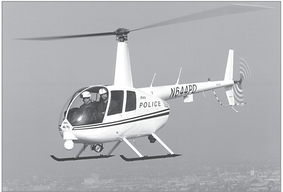
A WORK HORSE: The R44 Police Helicopter operates 100 hours between inspections, and 12 years or 2,200 hours between overhauls. It is the world's top-selling helicopter.
