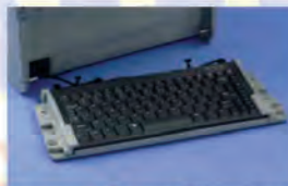
The integral keyboard detaches for ease of use in test subject data entry.
